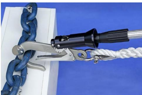
Attach the telescopic pole to the hook by screwing the pole in a clockwise direction. Then, by screwing the pole still further, the safety latch on the hook will open. Use the pole to unhitch the hook and line from the mooring and bring it back to the boat.
